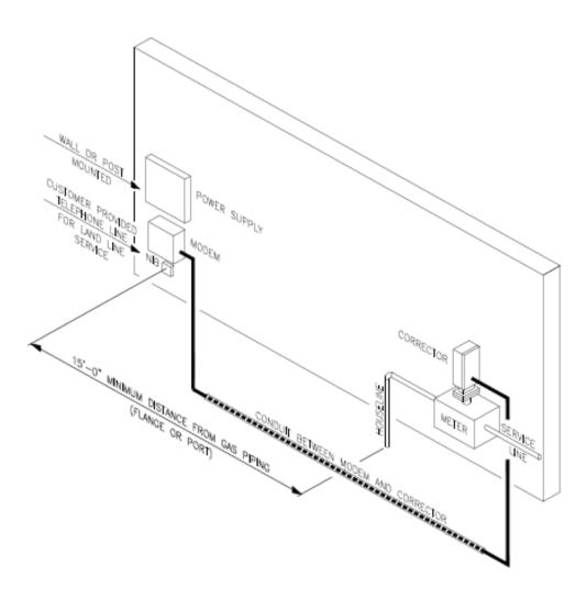
The 15 foot minimum distance referenced in the drawing above applies to equipment not rated for Class 1 Div 2 atmospheres. NEC/AGA guidelines for hazardous location installations should be followed.
